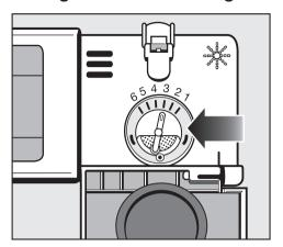
The dosage selector has settings from 1-6. It is set to "3" (3 ml) at the factory. Approx. 3 ml of rinse aid are then used per programme. This is a recommended setting.
